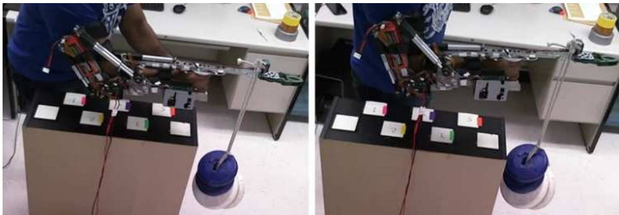
Figure 81: 17.85lb weight start and end point when moved with the eSARA platform.
