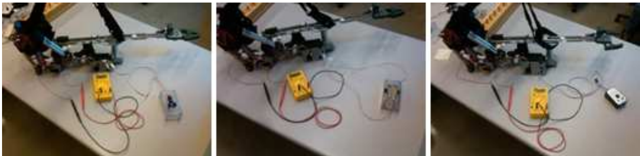
Figure 82: Current measuring experiment showing all the three modes, button, slider and voice control mode.
