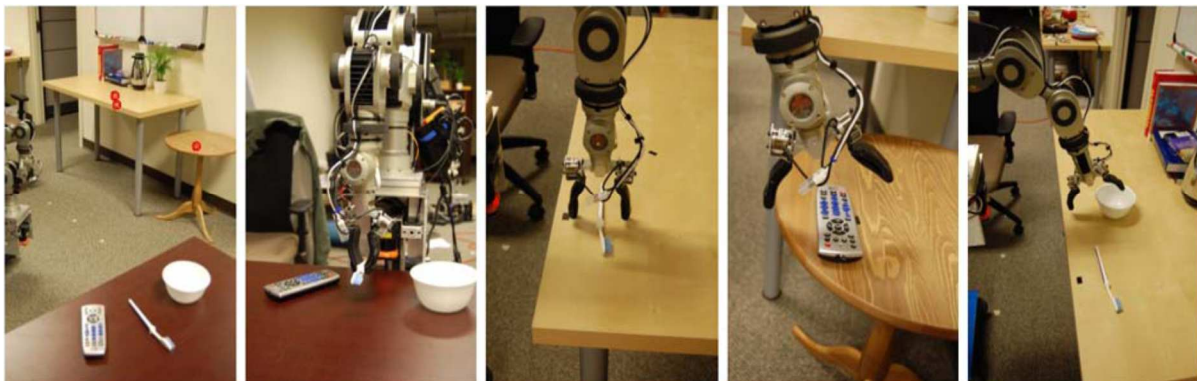
Figure 11: This figure shows the object placement experiment. The first image shows the three objects (TV remote, toothbrush and bowl) and the desired placement points (red circles). The second image shows the robot grasping the toothbrush, and the remaining three images show the robot placing the toothbrush, the TV remote, and the bowl [37-38].
