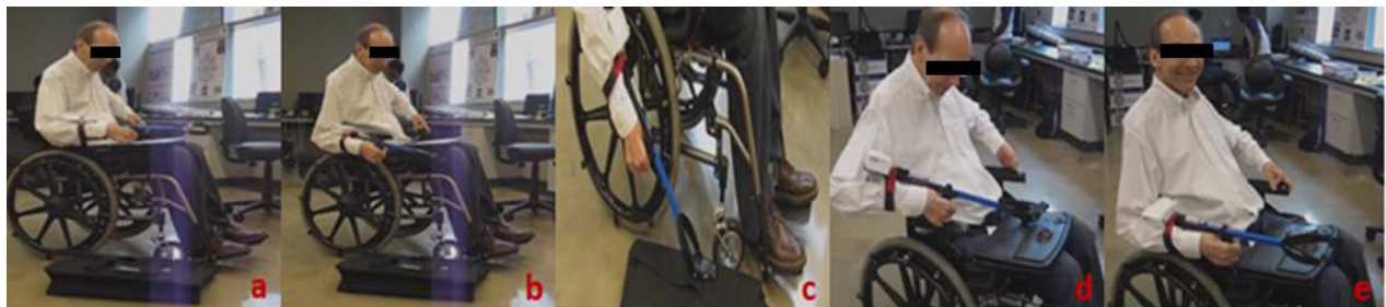
Figure 26: (a) Cell phone falls (b) SCI participant moves to pick up the cell phone using the reacher (c) Using voice commands the SCI participant controls gripper to secure the cell phone (d) SCI participant places the cell phone on his lap and then commands the gripper to open releasing cell phone (e) Success!
