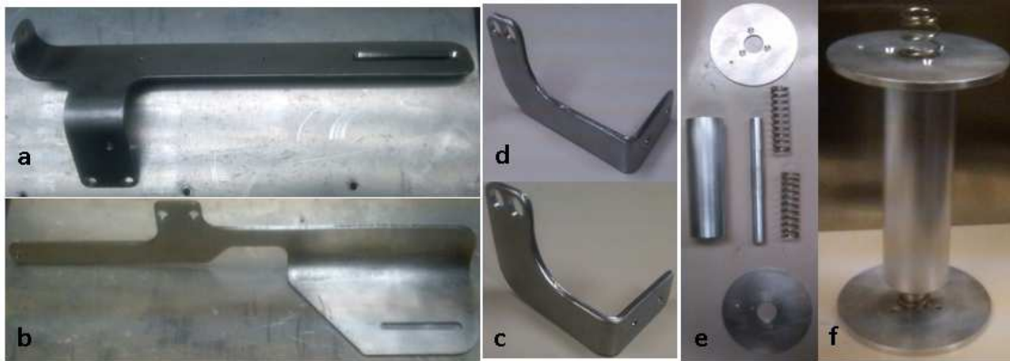
Figure 43: Machined parts of eSARA a) Top of the arm used to hold the extension rail, b) Bottom plate to hold the floating handle, c) Bracket to hold triceps actuator, d) Bracket to hold biceps actuator, e) Floating handle components, f) Assembled floating handle.
