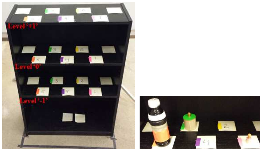
Figure 27: Left: Color coded test bench with three levels. Right: Test objects included a small peg (pink), larger peg (green), and a half pound bottle (orange).
