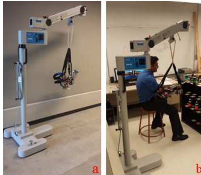
Figure 38: (a) Zeiss S21 [98] stand used to support eSARA's weight (b) user operating the Zeiss S21 system.
