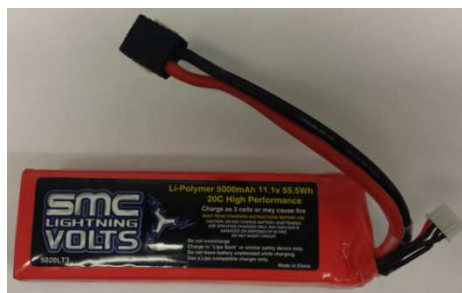
Figure 49: Lithium polymer battery: 11.1V, 55.5Wh with 5000mAh.
