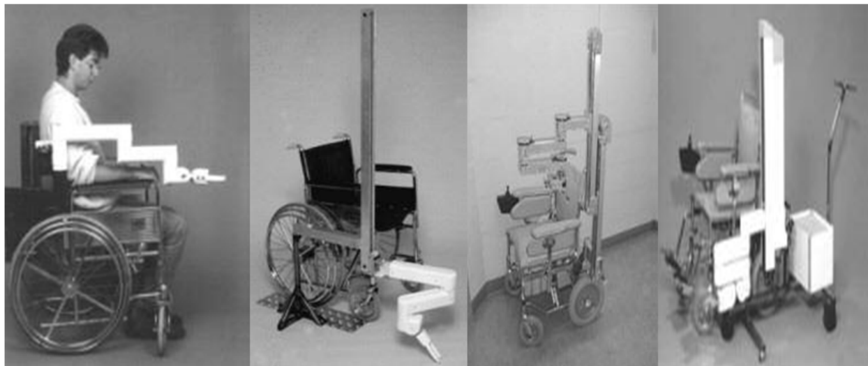
Figure 8: Different iterations of the wheelchair robotic arm [31-32].
